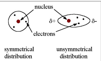
Because of the constant motion of the electrons, an atom or molecule can develop a temporary (instantaneous) dipole when its electrons are distributed unsymmetrically about the nucleus.
