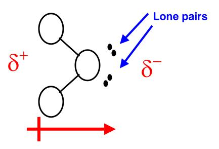
Another example of dipole-dipole interactions due molecular shape can be seen in ammonia (NH<sub>3</sub>):
