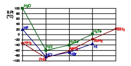
The high boiling points of water, hydrogen fluoride (HF) and ammonia ( $NH_3$ ) is an effect of the extensive hydrogen bonding between the molecules.
