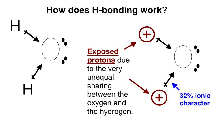
The hydrogen atom is very much exposed (naked) due to the unequal sharing with the oxygen. The naked proton is attracted to the lone pairs of electrons on other molecules. A temporary association of these two parts of adjacent molecules produces the hydrogen bond.
